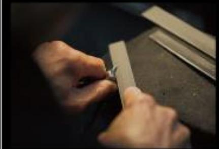
**8** Craftsmen adjusts the blades in increments of 1/1,000 millimeter for the perfect finish with no gap. Through these processes with the final inspection, our products become the best ones at last.
