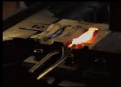
**2** A round rod heated to high temperature over 1,000 degrees is forged with 400 tons of pressure. The material is trained heavily. The craftsmen breathe new life into the steel.
