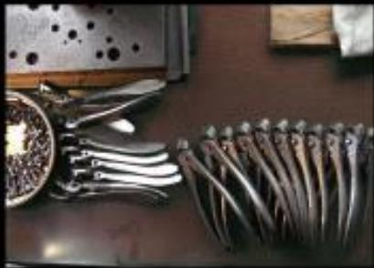
**5** The left and right parts cut out are riveted. Eventually they become the original "shape" of nail nippers.
